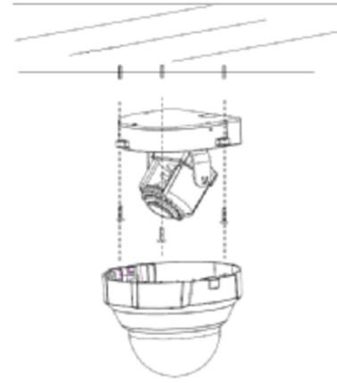
1. Paste install paper in the location you need , punch holes in the installation holes,push the rubber plug into the holes.
